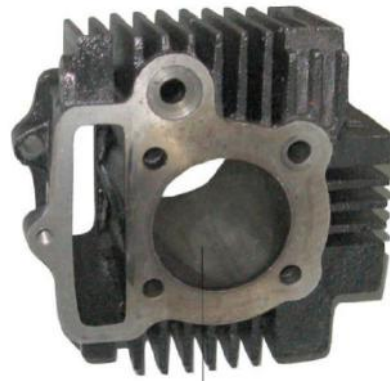
inner cylinder wall
